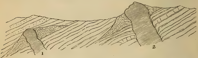
FIG. 285.—DIAGRAM-SECTION TO SHOW THE STRUCTURE OF OLD VOLCANIC VENTS, AND HOW THEY MAY BE CONCEALED AND EXPOSED.
